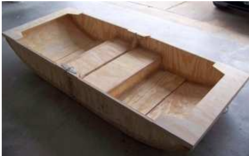
Unfinished Hull Assembled
