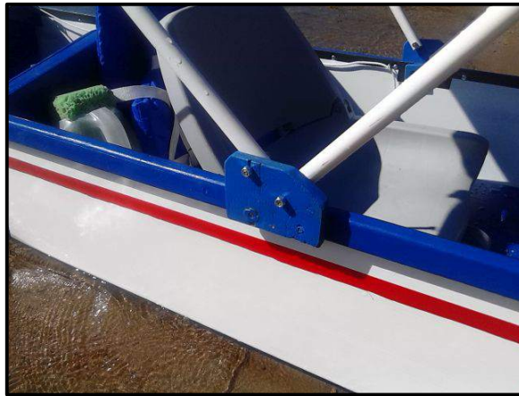
Top support assembly detail.
